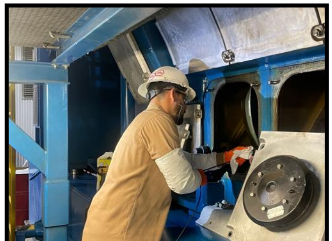
Jose Arriazola is performing Crankshaft Alignment Measurement.
